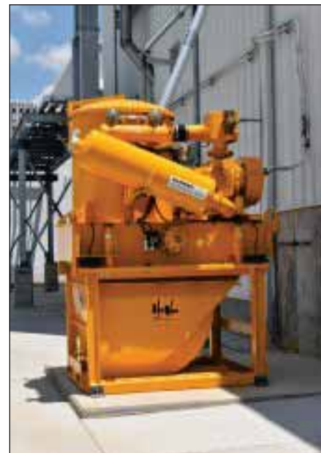
Above left: A special transition between pieces of equipment contains a spot filter for removing fines from the product flow. Above right: Hi-Vac vacuum systems powers cleanup throughout the plant. Below: Cleaver Brooks boiler is rated at 350 hp.
