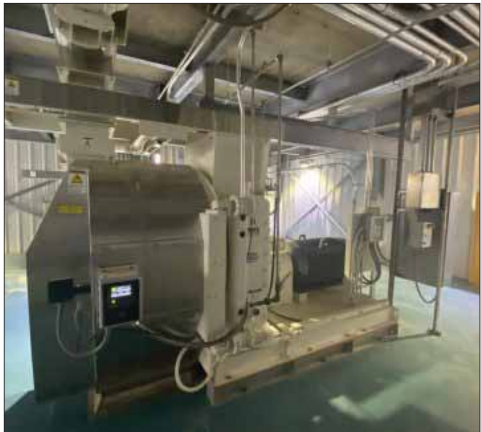
CPM Model 7932-12 pellet mill produces 30 tph.
